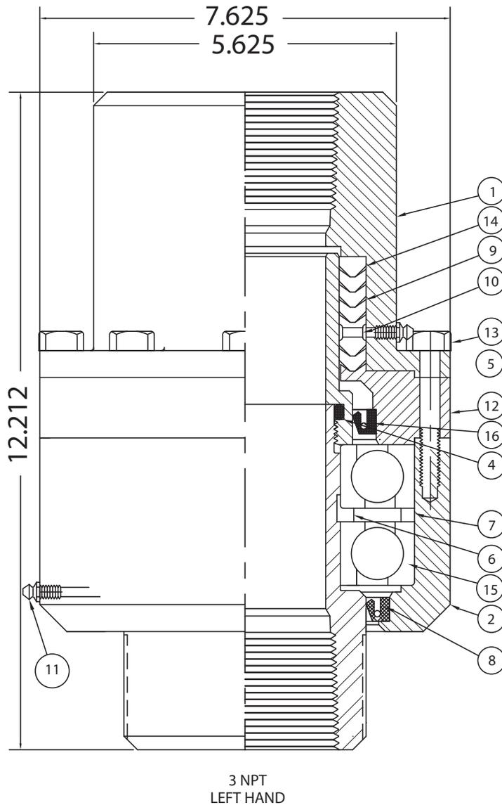
THE "J" SERIES OF SWIVELS ARE DESIGNED FOR MAXIMUM BORES FOR LARGE VOLUME OF AIR OR FLUID NEEDED ON TOP HEAD DRIVES.
